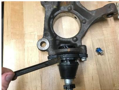
5. Install grease fitting and fill with grease.
